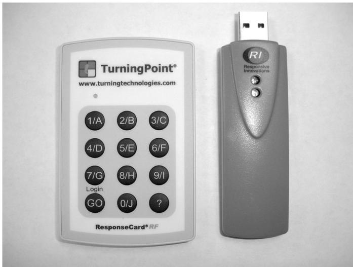
**Figure 1** Audience response hardware from TurningTechnologies: student transmitter (left) and instructor receiver (right)
